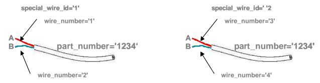
A special\_wire\_id specifies the identifier of the individual occurrence of multi-core wire. In contrast to the occurrence of a single wire which do not need to be identified in the module part list, each multi-core wire occurrence must be identified.
